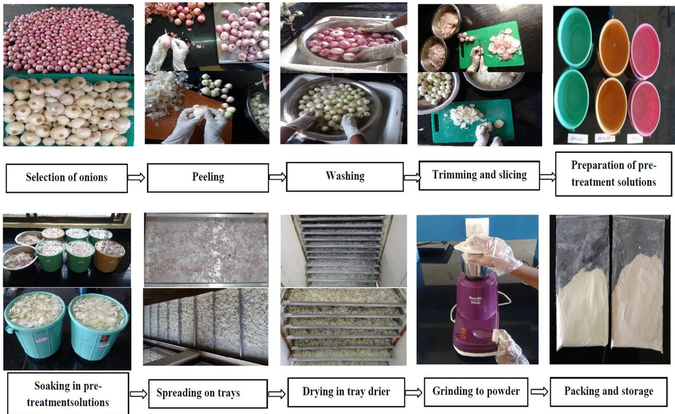
**Plate 1:** Sequence of operations in preparation of onion powder
