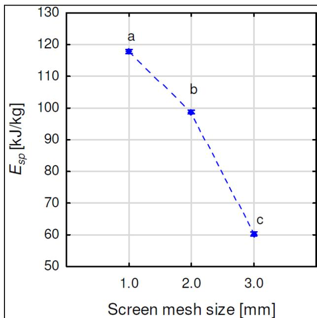
**Fig. 5 :** Influence of screen mesh size on the specific energy consumption
