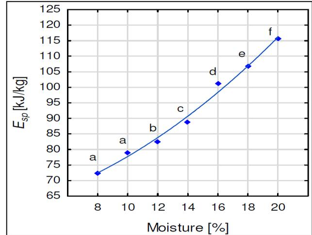
**Fig. 1 :** Influence of wheat moisture content on the specific energy consumption
