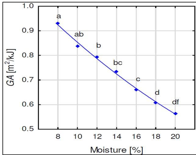
**Fig. 4 :** Influence of wheat moisture content on The grinding ability index
