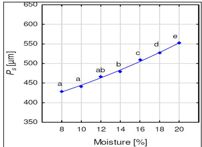
**Fig. 2 :** Influence of wheat moisture content on the mean particle size
