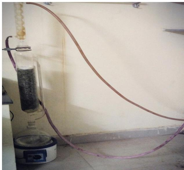
**Fig. 3:** Overall view of extraction using Soxhlet apparatus.
