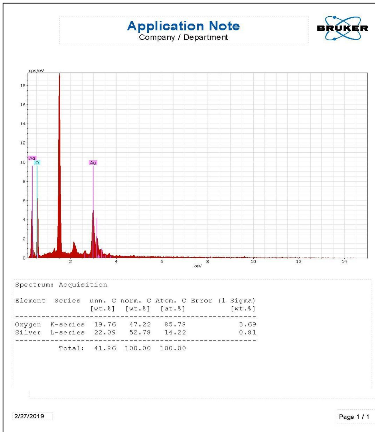
**Fig. 4:** Energy dispersive-x-ray spectroscopy analysis of Ag nanoparticles obtained by extract of the Ziziphus, appear strong signals of the silver and medium signal of Oxygen, the optical the weight percentage of silver (52.78%) and oxygen (47.22%).
