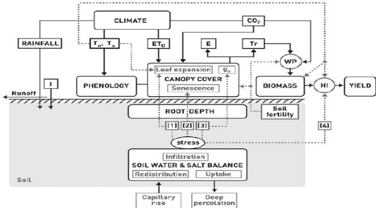
**Fig. 4 :** Chart of AquaCrop indicating the main components of the soil–plant–atmosphere continuum and the parameters driving phenology, canopy cover, transpiration, biomass production, and final yield [I, irrigation; Tn, minimum air temperature; Tx, Max air temperature; ET<sub>0</sub>, reference evapotranspiration; E, soil evaporation; Tr, canopy transpiration; g<sub>s</sub>, stomatal conductance; WP, water productivity; HI, harvest index (Steduto *et al.*, 2009).
