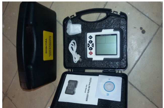
Picture 4: Shows how to set up the sensor used to measure carbon dioxide, temperature, relative humidity and dew point.
